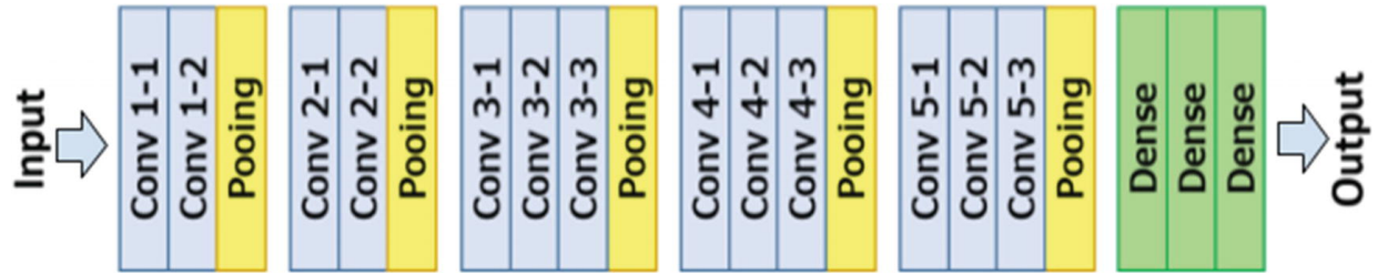
Figure 5-40 VGG-16 architecture with 16 layers (13 convolutional layers and 3 dense layers)
